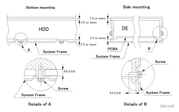
Figure 4.3 Mounting frame structure example
